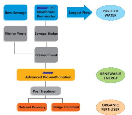
The ANDICOS design integrates state-of-the-art technologies like INDION IPC MBR and INDION Advanced Bio-methanation process to treat a combination of solid waste generated in sewage treatment process and organic kitchen waste generated in homes & communities.
